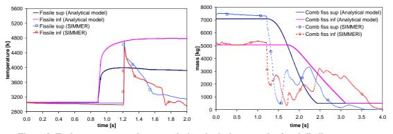
Figure 9: Fuel temperature and mass evolutions in the lower pools of each fissile zone - upper zone confined
