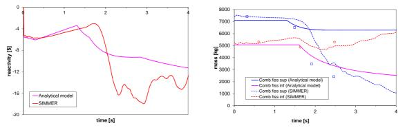
Figure 11: Reactivity and fuel mass evolutions with -5.49\$ of initial anti-reactivity and initial failure diameter 25cm.
