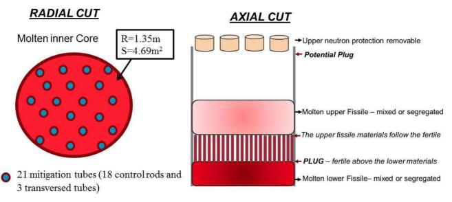
Figure 3: Considered initial degraded state (radial and axial cuts)
