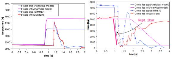
Figure 7: Fuel temperature and mass evolutions in the lower pool of each fissile zone (comb: fuel, sup:upper; inf:lower)<sup>6</sup>
