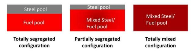
Figure 4: Various configuration of material repartition inside the upper or lower fissile zone.
