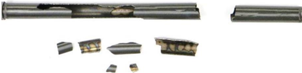
(a) Uncoated Zircaloy-4 clad segment, weight gain = 40,4 mg/cm 2
