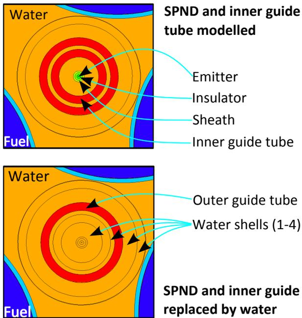
Fig. 2. Side views of a Rh SPND in the MP17 position in the computational model of the JSI TRIGA Mark II reactor. **Left:** SPND with materials explicitly modelled. **Right:** SPND with all materials replaced by water.
