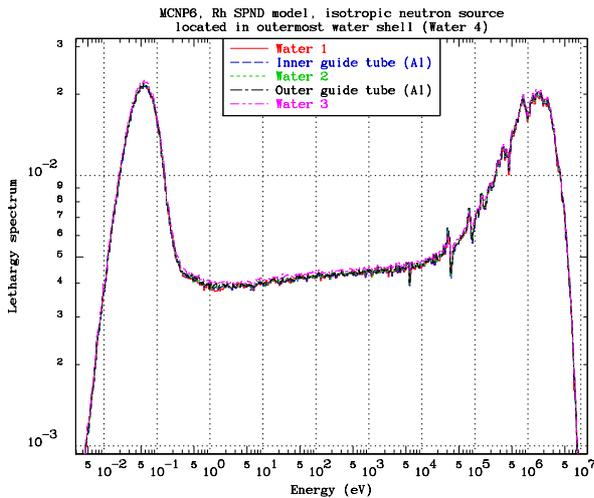
Fig. 6. Neutron spectra in the vicinity of a Rh SPND for a Step 2 calculation using an isotropic neutron source located in the outermost water shell (Water 4), with energy spectrum calculated in Step 1.
