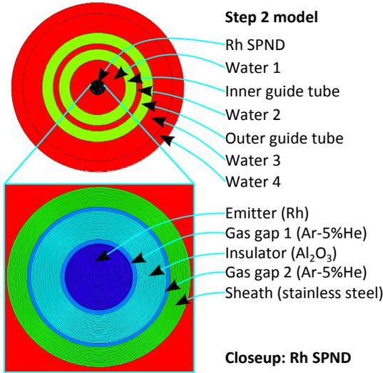
Fig. 5. Cross-section of the computational model used in Step 2 calculations. **Top:** whole model, **Bottom:** Rh SPND. The outside diameter of the outermost water shell is 31 mm.
