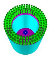
**Figure 1:** (color online) Cutouts to show the inside of a well counter. Polyethylene (magenta), Cadmium (cyan),
