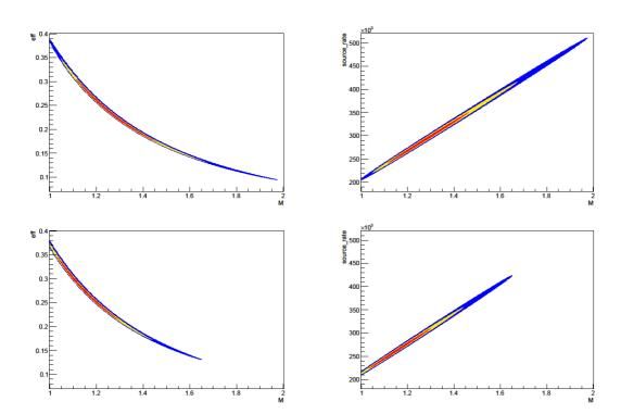
**Figure 2:** (color online) Credible regions for theoretical reconstructions of  $PuO_2$  ball: 68.27% (red), 95.45% (yellow), 99.73% (blue). Nuclear data for induced fission of <sup>239</sup>Pu at 1 MeV. The measurement time is equivalent to 350 seconds. Top left:  $(M, \varepsilon)$  with FREYA. Top right:  $(M, \overline{v}_{sp}F_s)$  with FREYA. Bottom right:  $(M, \overline{v}_{sp}F_s)$  without FREYA.
