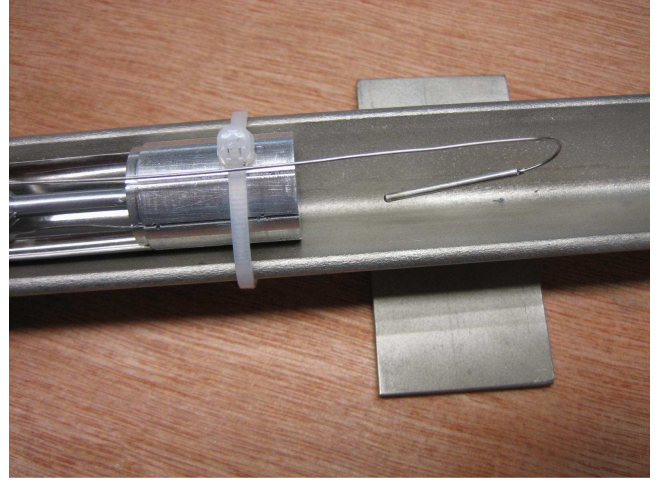
Fig. 9. Shaping and introduction of the specific Rhodium SPND inside central axis of the sample cell aluminum base. The emitter sensitive length is 10mm.
