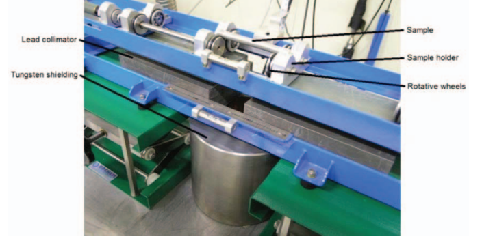
Fig. 1. Picture of the \gamma spectrometry bench with a 10-cm long sample.
