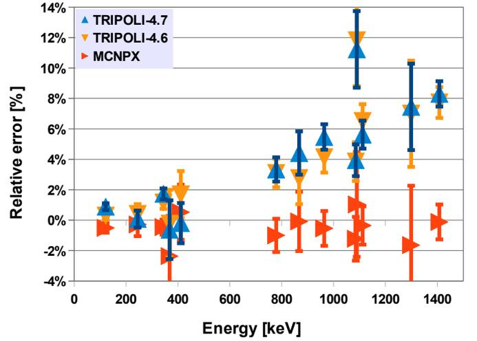
Fig. 3. First study. Relative error of TRIPOLI-4.6, TRIPOLI-4.7 and MCNPX simulated photopeaks of the  $^{152}\text{Eu}$  source simulated; MCNP5 is used as reference.
