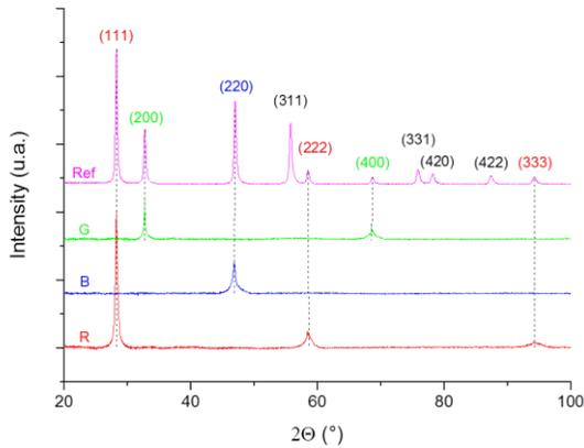
Figure 2. XRD pattern of the three  $\text{UO}_2$  single crystals for their major oriented surface after polishing, (100) surface for G sample, (110) surface for B sample and (111) surface for R sample. XRD pattern of  $\text{UO}_2$  powder as reference.
