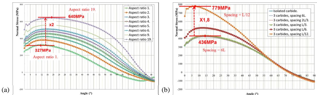
Figure 2: Distribution of normal stress along  $M_{23}C_6$  carbides / austenitic matrix interfaces after a creep time of 4166h involving a strain of 8% at 600°C and 220MPa, (a) effect of the carbide aspect ratio, (b) effect of the inter-carbide spacing for an aspect ratio of 3.
