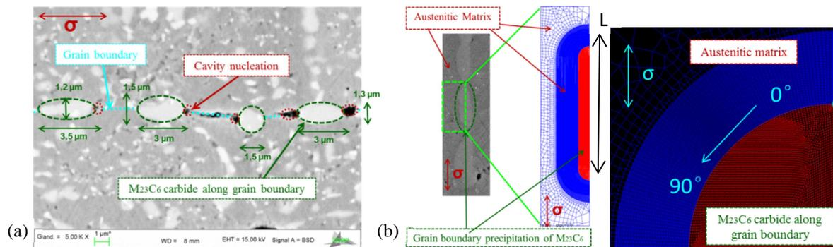
Figure 1: (a) FEG-SEM image, creep test, longitudinal section, 700°C, 100MPa, 2226h. (b) Mesh of a  $M_{23}C_6$  carbide embedded in an austenitic matrix and mesh refinement along the carbide interface. The loading direction is vertical. The carbide length is expressed as  $L$ .
