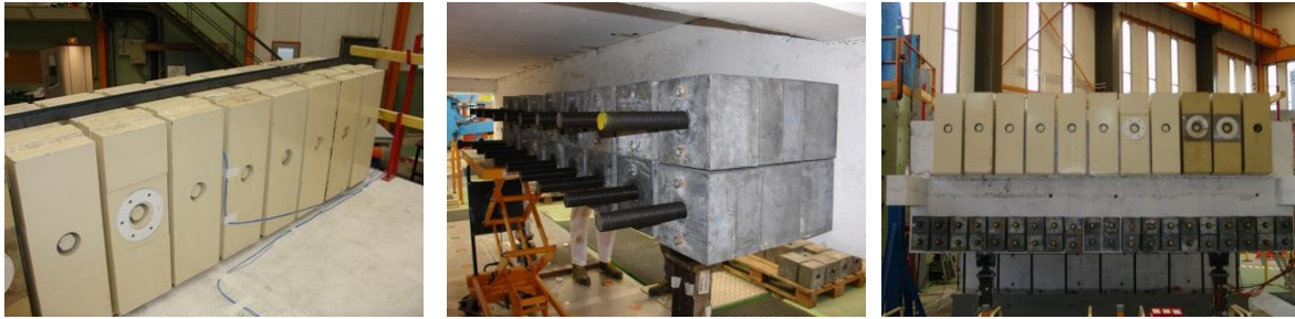
Figure 3: Additional masses fixed on Model-2
