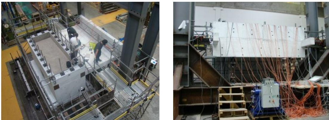
Figure 4: Static cyclic test set-up (Model-1)
