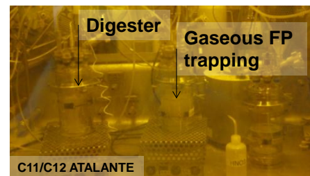
Fig. 8. View of the experimental setup used to digest dissolution-resistant solid residues containing some plutonium (ATALANTE C11/C12 shielded cells).
