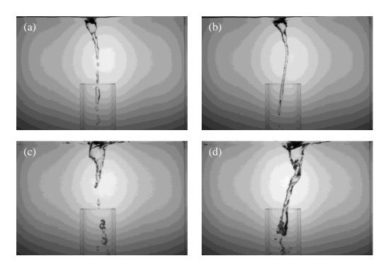
Figure 2. Snapshot of non-continuous surface swirls and gas entrainments for (a)  $Q_{in} = 5.7 \text{m}^3/\text{h}$ ,  $Q_{suction} = 4.9 \text{m}^3/\text{h}$  and (c)  $Q_{in} = 9.5 \text{m}^3/\text{h}$ ,  $Q_{suction} = 7.1 \text{m}^3/\text{h}$ . Snapshot gas entrainment trough Continuous Surface swirls for (b)  $Q_{in} = 5.7 \text{m}^3/\text{h}$ ,  $Q_{suction} = 4.9 \text{m}^3/\text{h}$  and (d)  $Q_{in} = 9.5 \text{m}^3/\text{h}$ ,  $Q_{suction} = 7.1 \text{m}^3/\text{h}$ .
