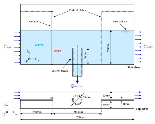
Figure 1. Experimental set up. The origin of the Cartesian frame is set on the border of the vertical plate at the height of the suction nozzle. The x-axis coincides with the horizontal main flow, y and z axis are respectively horizontal and vertical.
