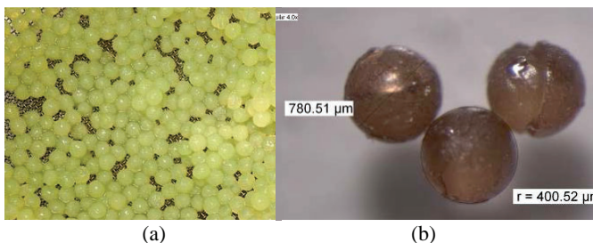
Fig. 8. Spheres collected after microwaved gelation before (a) and after (b) drying.
