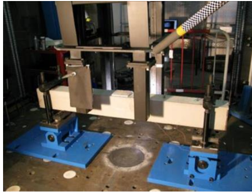
Figure 3: View of a beam with its two rotating bearings instrumented with load cells.
