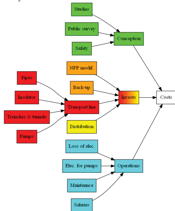
Fig. 3. Cost breakdown structure
