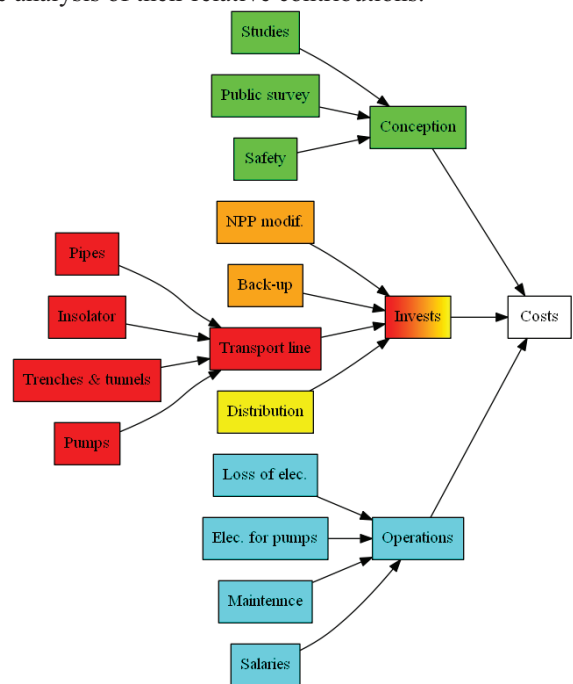
Fig. 3. Cost breakdown structure
