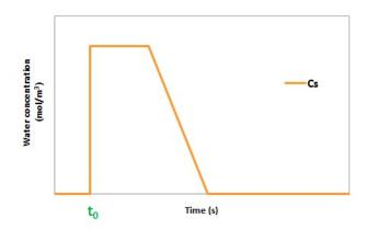
Figure 4 : Ideal breakthrough curve of water (t<sub>0</sub> represents the beginning of the experiment)
