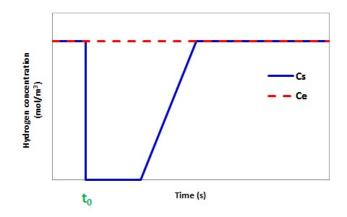
Figure 3 : Ideal breakthrough curve of hydrogen (t<sub>0</sub> represents the beginning of the experiment)
