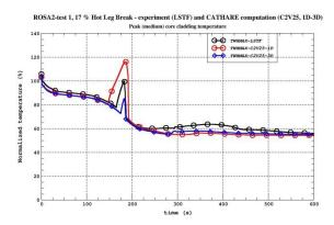
Figure 10. Temperature in the core rod
