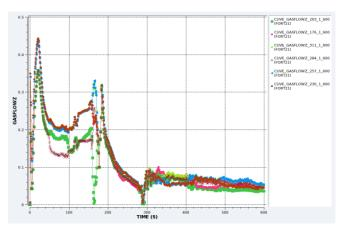
Figure 13. Gas flowrate vs time. Curves correspond to the different sectors (1 to 6) in the second crown (the middle one) at about 5 m from the bottom of the PV
