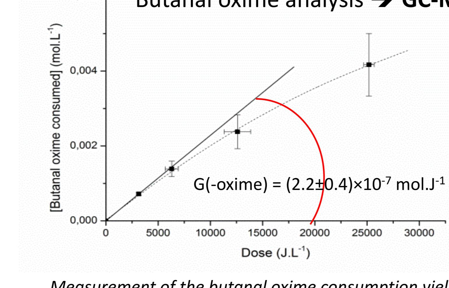
Measurement of the butanal oxime consumption yield by irradiation of aqueous solution of  $10^2 \text{ mol.L}^{-1}$  butanal oxime.
