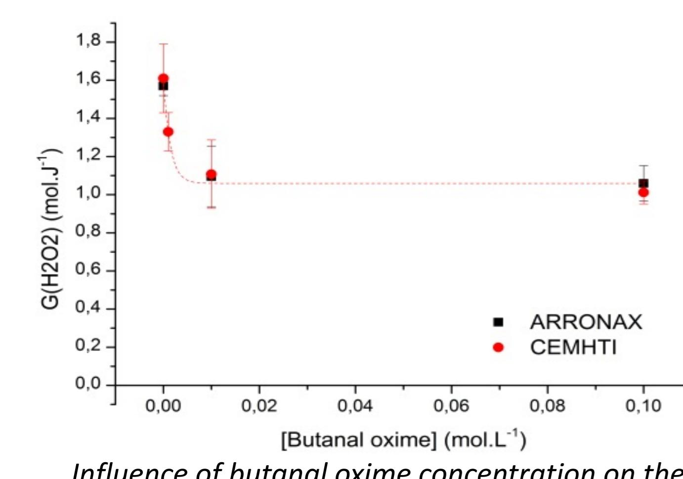
Butanal oxime inhibits  $\text{H}_2\text{O}_2$  production→ Scavenging of  $\cdot\text{OH}$
