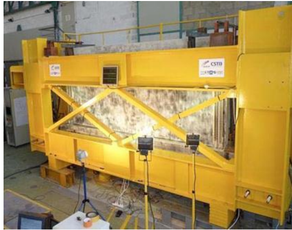
Figure 8: Shear wall experimental setup [14]
