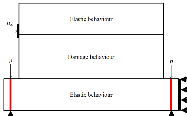
Figure 12: Loading and boundary conditions
