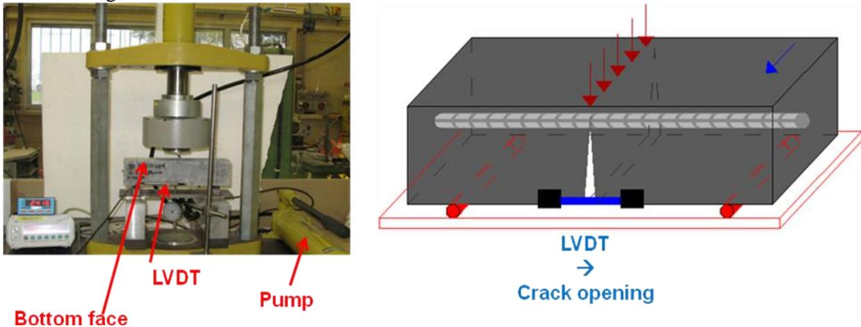
Figure 4: Three point bending test on  $70 \times 70 \times 280$  mm<sup>3</sup> specimen
