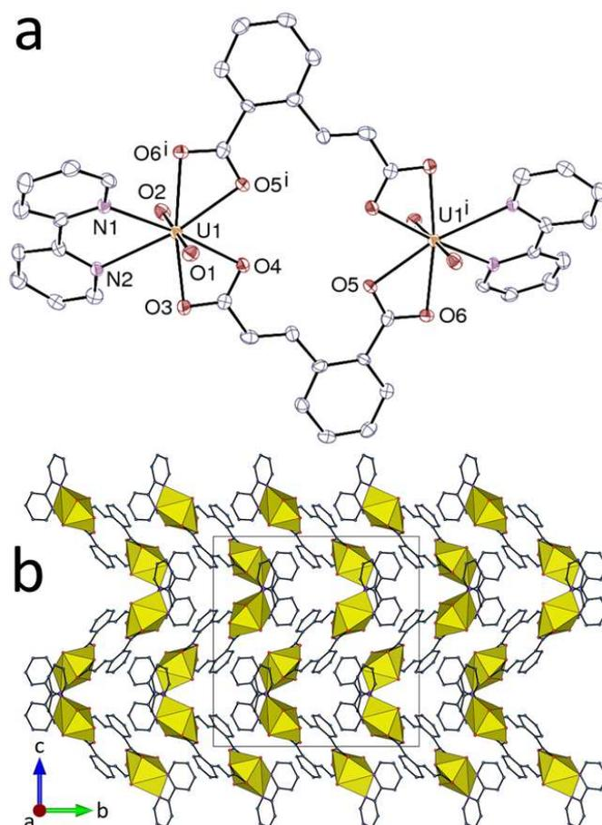
**Figure 3.** (a) View of compound **3**. Displacement ellipsoids drawn at the 50% probability level and hydrogen atoms are omitted. Symmetry codes:  $i = 1 - x, 1 - y, 1 - z$ . (b) Packing showing uranium coordination polyhedra.
