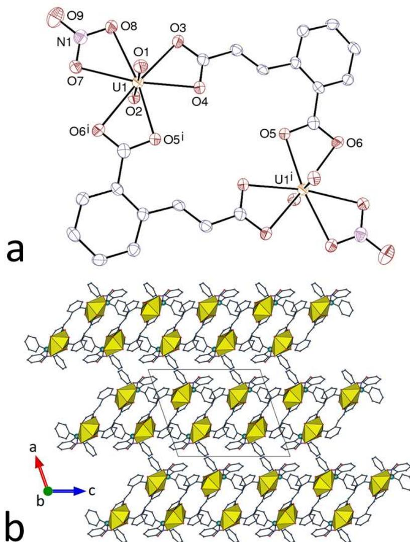
**Figure 1.** (a) View of compound **1**. Displacement ellipsoids drawn at the 50% probability level. Counterions and hydrogen atoms are omitted. Symmetry code:  $i = 1 - x, 2 - y, 1 - z$ . (b) Packing with uranium coordination polyhedra colored yellow.
