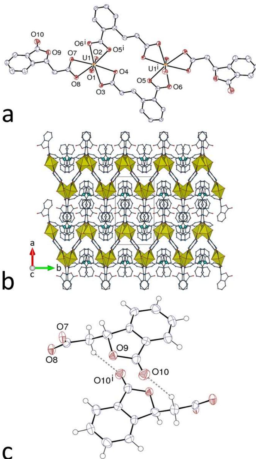
**Figure 2.** (a) View of compound 2. Displacement ellipsoids drawn at the 50% probability level. Counterions and hydrogen atoms are omitted. Symmetry code:  $i = 2 - x, 1 - y, 2 - z$ . (b) Packing showing uranium coordination polyhedra. (c) Dimerization of dibf<sup>-</sup> ligands through CH...O hydrogen bonding (dashed lines). Symmetry code:  $i = 1 - x, 2 - y, 2 - z$ .
