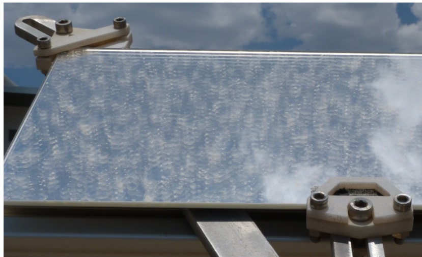
Figure 3. Sample surface after a strong soiling event, showing an inhomogeneous soiling pattern.
