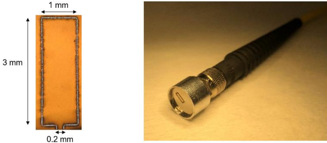
Figure 4. On the left, microscope view of the 3 mm x 1 mm cantilever beam with the 100 \mu\text{m} x 200 \mu\text{m} hinge (bottom). On the right, membrane assembled on the SMA optical fiber.
