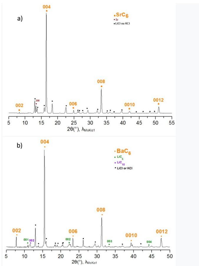
**Fig.1 00/ X-ray diffraction patterns ( $\lambda_{\text{MoK}\alpha 1} = 70.926$  pm) of the first stage GIC a) SrC<sub>6</sub> ( $l_c = 494$  pm) and b) BaC<sub>6</sub> ( $l_c = 525$  pm)**
