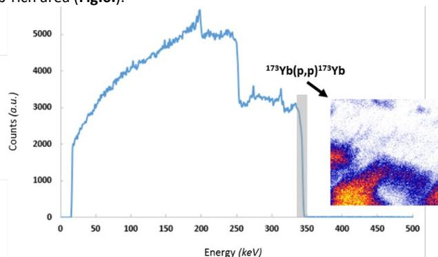
Fig 6. Spectrum of the YbC<sub>6</sub>-containing sample. The grey area indicates the energy windows considered to draw contrast maps of ytterbium.
