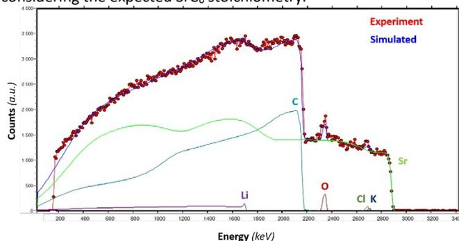
**Fig.2. Recorded RBS/NRA spectrum of the Sr-based GIC synthesized by the molten salts method and its simulation. Each individual elementary contribution to the simulation is drawn. Red spots: experiment; blue solid line: simulation.**
