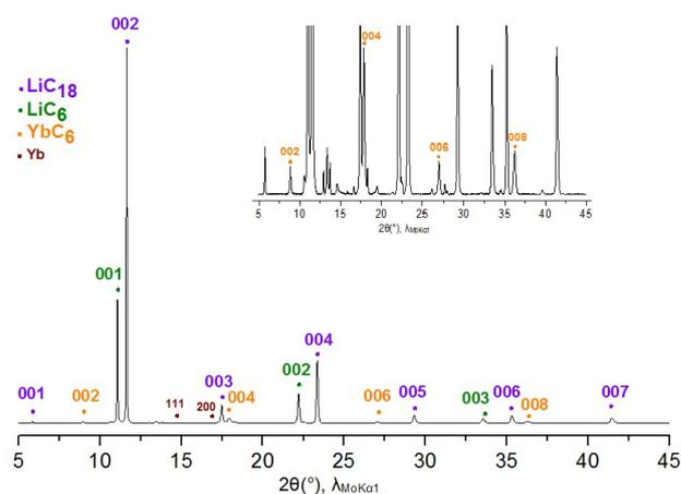
**Fig.4.** 00/ X-ray diffraction pattern ( $\lambda_{\text{MoK}\alpha 1} = 70.926 \text{ \AA}$ )  $\text{YbC}_6$ -containing sample. The zoom is referred to  $\text{YbC}_6$  reflections
