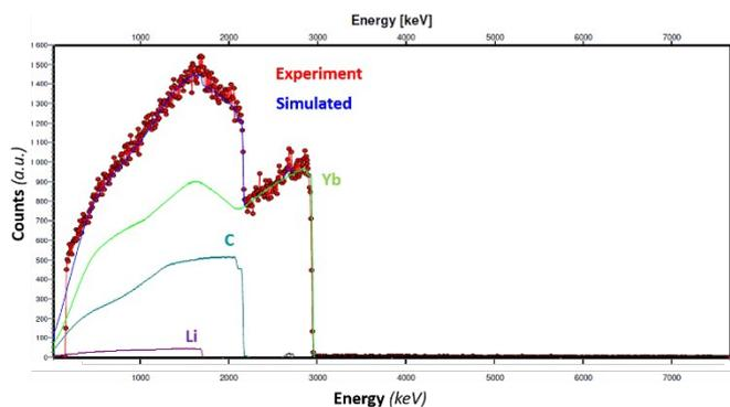
Fig.7. Recorded RBS/NRA spectrum of the YbC<sub>6</sub>-containing sample synthesized by the molten salts method and its simulation. Each individual elementary contribution to the simulation is drawn. Red spots: experiment; blue solid line: simulation.
