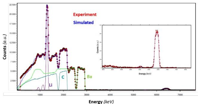
**Fig.3.** Recorded RBS/NRA spectrum of the Ba-based GIC synthesized by the molten salts method and its simulation. Each individual elementary contribution to the simulation is drawn. Red spots: experiment; blue solid line: simulation. The inset is focused on the  $^7\text{Li}$  nuclear reaction energy range.
