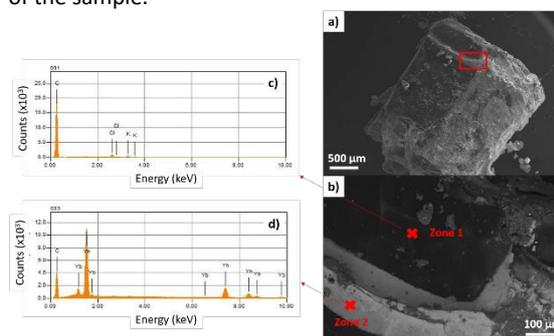
**Fig. 5.** a) SEM micrograph (secondary electrons imaging) of the  $\text{YbC}_6$ -containing sample b) SEM micrograph (backscattered electrons imaging) of the framed zone c) EDX spectrum on zone 1 d) EDX spectrum on zone 2.
