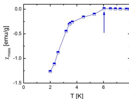
Fig.8. Low temperature ZFC mass susceptibility  $\chi_m$  of the YbC<sub>6</sub>-containing sample taken under an external field of 1 mT. The arrow indicates the superconducting critical temperature  $T_C$ .
