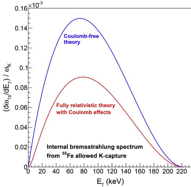
**Fig. 1.** Internal bremsstrahlung spectrum from  $^{55}\text{Fe}$  allowed K capture. The blue spectrum has been calculated using Coulomb-free theory (Morrison and Schiff, 1940). The red spectrum has been calculated by means of the fully relativistic theory from (Martin and Glauber, 1958). (For interpretation of the references to colour in this figure legend, the reader is referred to the Web version of this article.)
