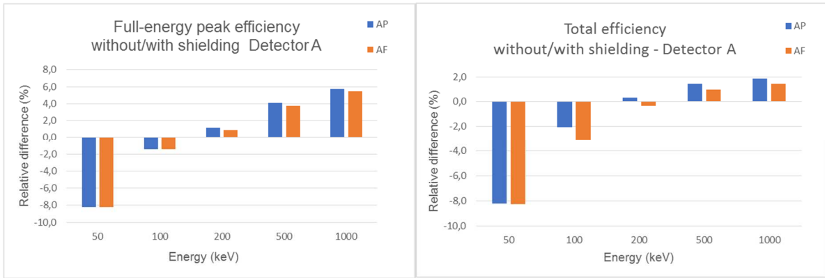
Figure 5: Relative difference between full-energy peak efficiencies for detector A with point and filter sources calculated by MCNP, with and without the lead shielding.
