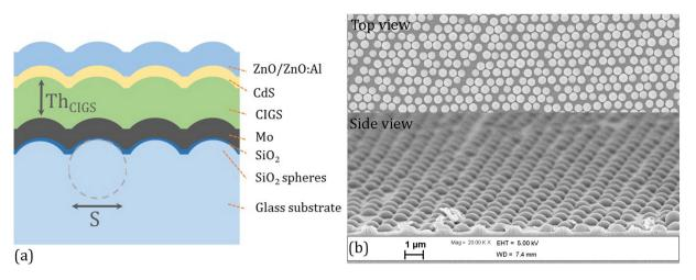
**Fig. 1.** (a) Schematic view of the solar cells structure used in this study. Dashed line is a guide for the eye to represent spherical particle after integration into the glass substrate. Parameters of the study (dimension of the texturation imposed by sphere size (S) and thickness of CIGS absorber layer (Th<sub>CIGS</sub>)) are depicted as well. (b) Scanning Electron Microscopy (SEM) top and side views of textured glass substrates with 1 µm diameter buried spheres (S-1.0).
