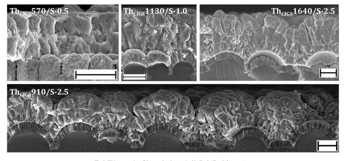
Fig. 6. SEM cross section of the samples characterized in Fig. 5. All scale bars are 1  $\mu$ m.
