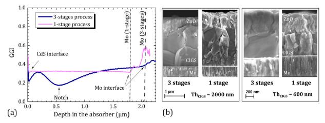
Fig. 2. (a) GGI profiles as function of absorber depth for 3-stages and 1 stage processes measured by GDS on flat substrates. CdS and Mo interfaces as well as notch position are indicated for clarity. (b) SEM cross section of CIGS solar cells on reference flat substrates with a SiO<sub>2</sub> barrier.
