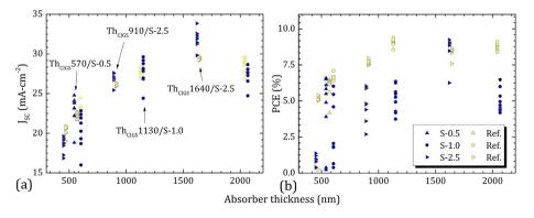
**Fig. 4.** (a) J<sub>SC</sub> and (b) PCE of the 1-stage process CIGS solar cells fabricated on reference substrates (yellow) and textured substrates (blue) for different texturation sizes (S). Data points for textured samples have been a little bit x-translated for greater clarity. Comments in the J<sub>SC</sub> graph are reference to the EQE measurements (Fig. 5). (For interpretation of the references to colour in this figure legend, the reader is referred to the web version of this article.)
