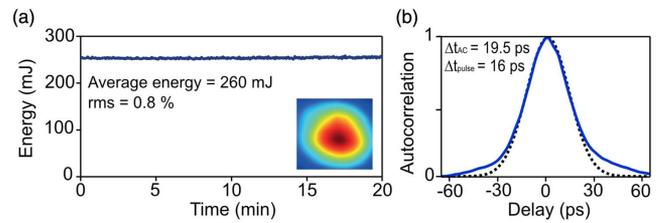
**Fig. 2.** (a) Measured stability at full power from the Ho:YLF pump system. The inset shows the beam profile measured at full power. (b) Measured intensity autocorrelation (blue) of the 2052 nm pump pulses after compression in the dielectric-coated gratings, together with a Gaussian fit (dashed black). The FWHM duration of the autocorrelation signal was measured to be 19.5 ps corresponding to a pulse duration of 16 ps at FWHM.
