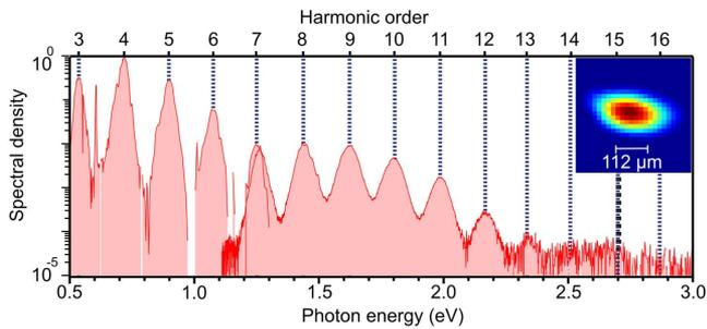
**Fig. 5.** Measured high-harmonic spectrum in bulk ZnSe crystal (red curve) and the harmonic orders from the third to 13th harmonic, both even and odd, shown in dashed blue lines. The black thick dashed line refers to the bandgap of the crystal. The inset shows the measured beam profile of the 7  $\mu\text{m}$  pulses at the generation plane of the harmonics.
