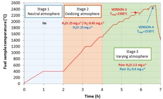
Fig. 1. Thermal sequence of the VERDON-3 and 4 tests.
