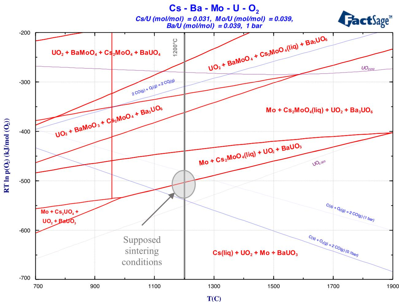
**Fig. 11.** Predominance diagram for the U-Cs-Ba-Mo-O<sub>2</sub> system (Batch 8), considering the quantities of elements added before sintering, obtained using the SGPS database of FactSage [3,4].
