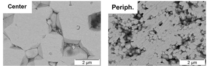
**Fig. 7.** SEM-BSE images showing the morphology of the grains in the centre (left) and the periphery (right) of the pellets of batch 3 (UO<sub>2</sub> + 1.2% Cs<sub>2</sub>U<sub>x</sub>O<sub>y</sub>).
