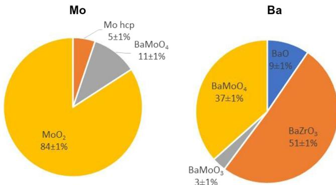
**Fig. 6.** Linear combination fitting results performed between  $-20$  and  $+60$  eV around Mo K-absorption edge and Ba L<sub>3</sub>-absorption edge of the O1000 sample.
