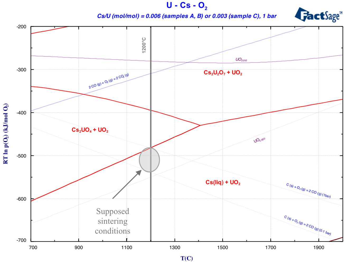
**Fig. 9.** Predominance diagram for the Cs-U-O<sub>2</sub> system (Batch 3), considering the quantities of elements remaining in the system after sintering (obtained using the SGPS database of FactSage [3,4]).
