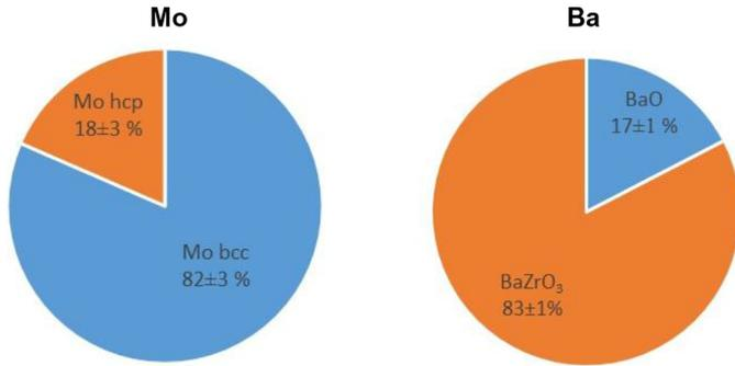
**Fig. 5.** Linear combination fitting results performed between  $-20$  and  $+60$  eV around Mo K-absorption edge and Ba L<sub>3</sub>-absorption edge of the T<sub>0</sub>(SIMF) sample.
