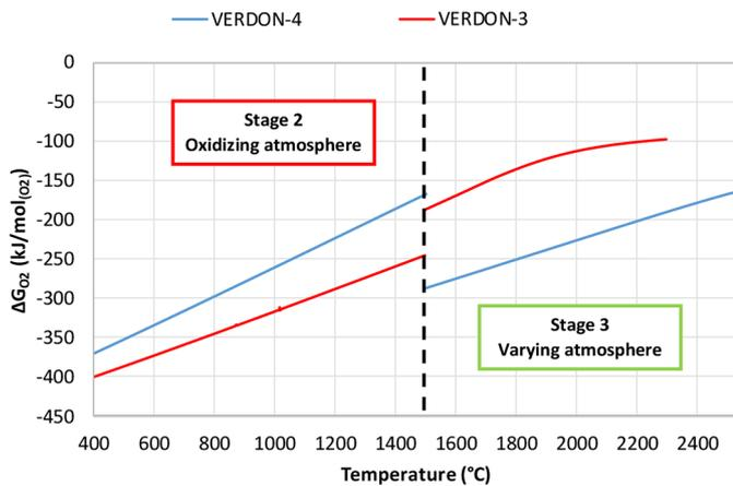
**Fig. 2.** Evolution of the oxygen potential during the stage 2 and 3 of the VERDON-3 and 4 tests, calculated from the H<sub>2</sub>O/H<sub>2</sub> system using Thermo-Calc [1] coupled with the TAF-ID [2].
