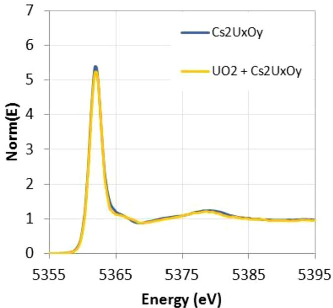
**Fig. 8.** Experimental HERFD-XANES spectra of Cs<sub>2</sub>U<sub>x</sub>O<sub>y</sub> standard and a sample of batch 3 as-sintered acquired on the FAME-UHD beamline (ESRF).
