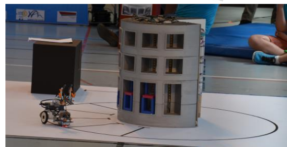
Figure 7. Picture of the TRANSPORT challenge. The robot must autonomously follow the tracks plotted on the floor and pick a brick (here in red) in each “port” of the ITER mock-up (in the middle). Once got, the robot must bring back the brick to the “hot-cell” (black zone at the left of the figure).
