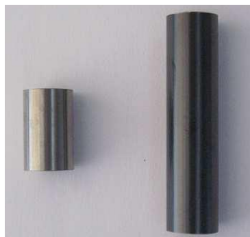
Figure 1: left: new Zircaloy-4 clad; right: oxidized clad with thin layer of black color oxide.
