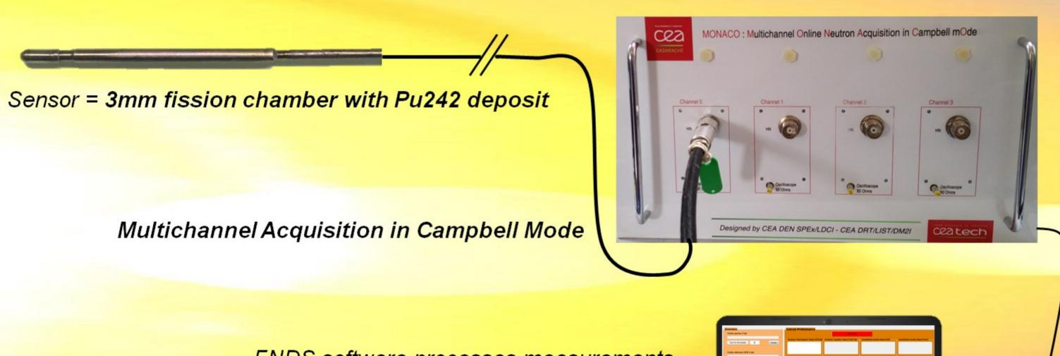
While most fission chambers are primarily used for thermal neutron detection, the CEA and the SCK•CEN have jointly developed and patented the first and unique acquisition system able to provide an online measurement of the fast neutron flux (E>1MeV) in typical MTR conditions, where overall neutron flux level can be as high as 10<sup>15</sup> n.cm<sup>-2</sup>.s<sup>-1</sup> and is generally dominated by thermal neutrons, and where high gamma flux can disturb fission chamber measurement.
