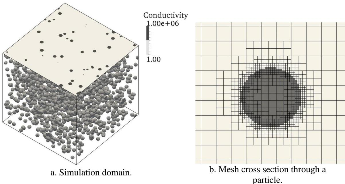
Figure 2. Simulated dispersion of volume fraction 6%.
