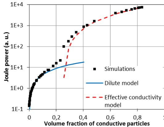
Figure 5. Normalized Joule power induced in the dispersion.
