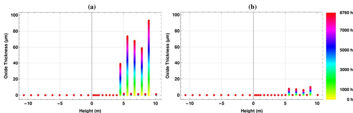
Figure 9. Apparent thickness of iron oxide on a SG tube as a function of the height in the SG (a) without PAA and (b) with 13 μg.kg<sup>-1</sup> of ligand. Operating time ranges between 0 and 8760 h (see the legend) *i.e.* one year of nominal operating conditions
