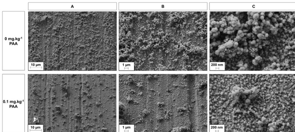
Figure 5. SEM-secondary electron images of the tube surface in the liquid free span after the reference test and the test containing 0.1 mg.kg<sup>-1</sup> PAA
