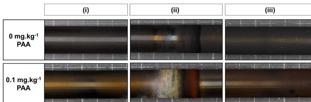
Figure 3. Photograph of the (i) humid vapour section, (ii) liquid/vapour interface section and (iii) liquid section of the IRIS tube after testing at 0 and 0.1 mg.kg<sup>-1</sup> PAA
