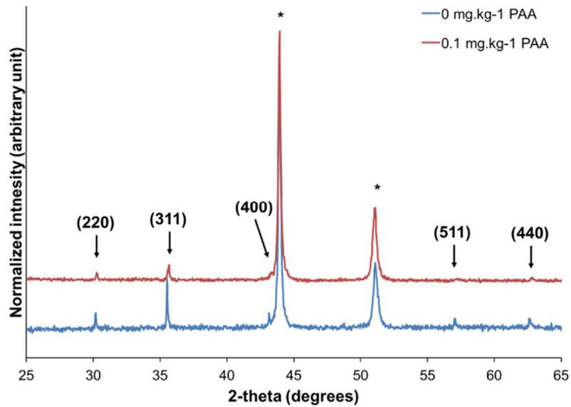
Figure 4. X-ray Diffraction pattern for the IRIS tube at the liquid free-span section (Figure 2 (iii)), deposited in the presence and absence of PAA. The \* indicates peaks corresponding to Inconel 690TT, (CuK $\alpha$  radiation = 1.5418 Å)
