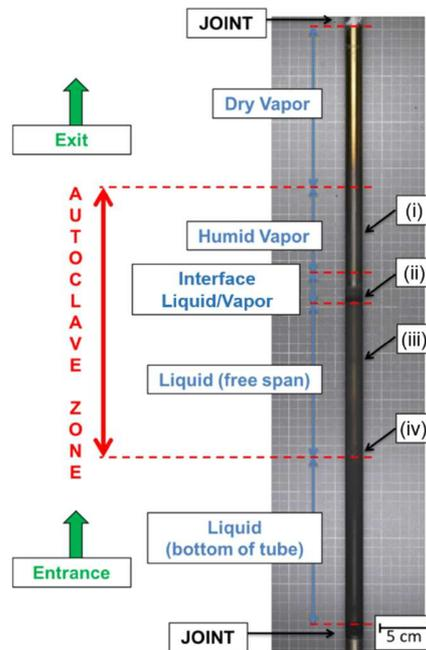
Figure 2. Sections of IRIS tube analysed by SEM and XRD
