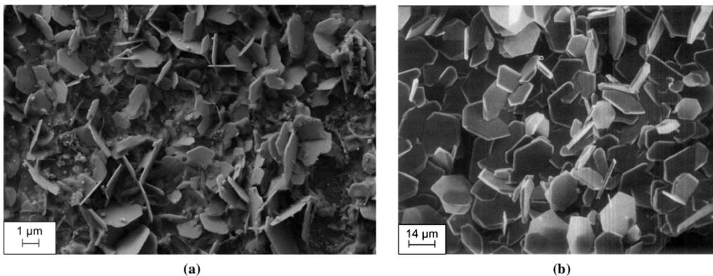
Figure 7. SEM-secondary electron images of (a) liquid/vapor interface section after testing at 0.1 mg.kg<sup>-1</sup> PAA in IRIS and (b) pure hematite produced by hydrothermal growth in the work by SAPIESZKO & MATIJEVIĆ (1980)
