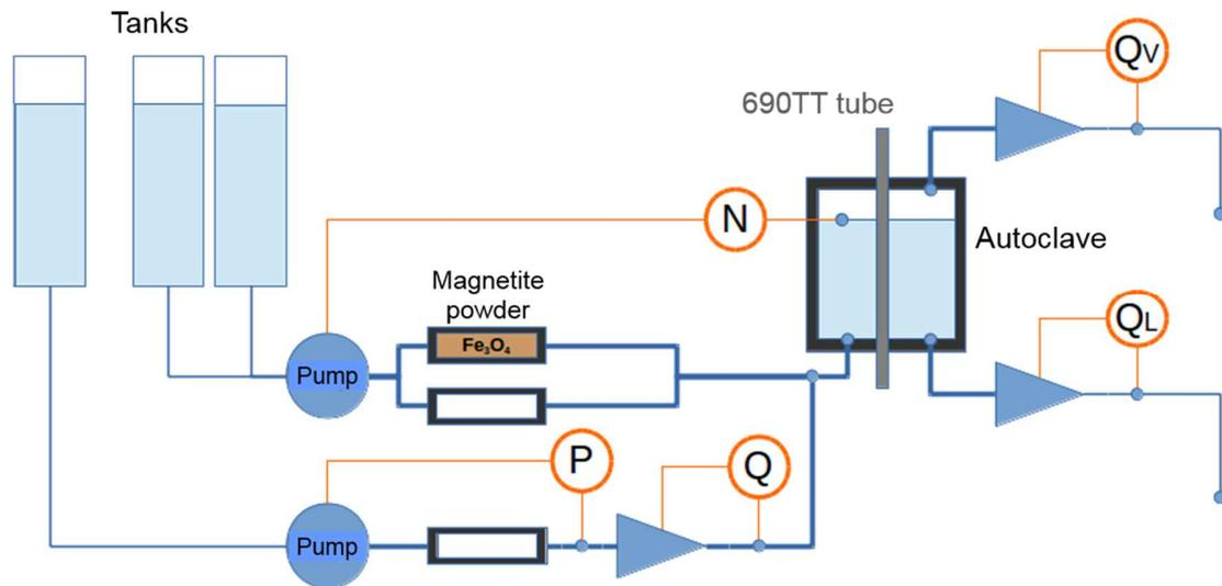
Figure 1. Simplified scheme of the setup named IRIS (for Research Instrumentation for the Investigation of Speciation in aqueous media at high temperature) ROY, BLANCHARD, MERTENS, & YOU (2014).
