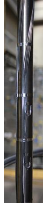
Figure 5 : Electrical rod with thermocouples clamped on the cladding
