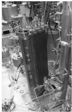
Dissolution of spent nuclear fuel and filtration of the solution
