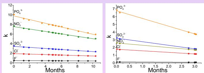
→ Linear decrease of retention factors as a function of the operating time of the Cap-IC columns whatever the type of columns and the studied anions
