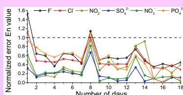
→ Accurate quantification of all anions by using the same calibration curve during 18 days
