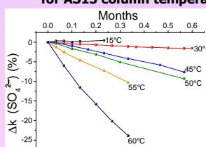
→ Application of a limited column temperature (<20°C) when no analysis is performed in order to preserve the Cap-IC column retention capabilities at long term
