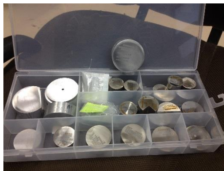
15 samples of 3 matrices (Fe, Ni, Ti)
