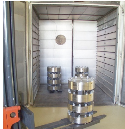
Figure 3: Test principle: Left side – mockup under the press. Right side – mockups piled up inside a furnace
