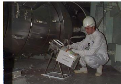
EMECC device Measurement of a PWR hot leg
