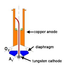
Figure 3: Schematic view of the torch.
