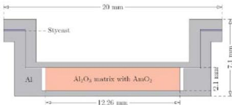
**Fig. 3.** Drawing of JRC-IRMM americium samples
