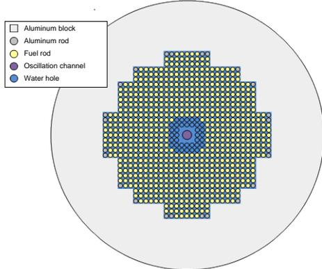
**Fig. 1.** Drawing of the AMSTRAMGRAM experimental zone.
