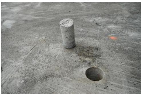
Core made of concrete containing C-14
