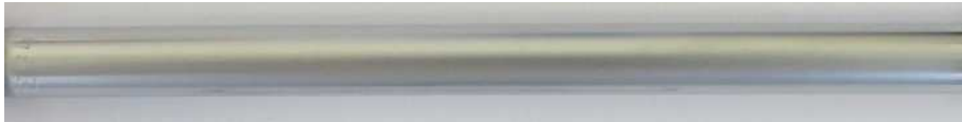
SRA Low-Tin Zircaloy-4 from AREVA-NP 50cm clad segments with ~15 \mu m thick Cr coating
