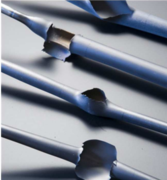
Uncoated claddings appearance after ballooning and burst (« EDGAR ») testing
