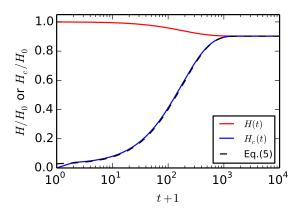
**Figure 2.** Height of the modeled packing H(t) (red curve) normalized by the initial height  $H_0$ , height of the compacted grains  $H_c(t)$  (blue curve), compared with expression 5 (black dashed line). The model parameters are N = 250,  $\phi_0 = 0.9$  from an average of 20 000 runs.
