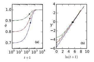
**Figure 3.** Simulation results (colored continuous lines) for N = 250 grains, averaged on 20 000 runs. Each curve is fitted by Eq. 1 (dashed black line) (a) Compaction curves for three different initial conditions. The star symbols indicate the inflexion points at time t = T, (b) Same data in the (ln t, Y) space.
