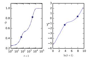
**Figure 4.** Simulation result for a modeled cohesive granular material. The parameters are N = 1250, n = 50,  $\phi_{0c} = \phi_{0g} = 0.5$ . (a) volume fraction as a function of time in a log-lin space (blue curve) and the fitted expression (12) (black dashed line). The stars indicate the  $T_c$  and  $T_g$  characteristic times. (b) Same data plotted as  $Y = \ln(\ln(1/C))$  as a function of  $\ln t$ .
