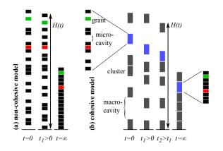
**Figure 1.** (a) Sketch of the non-cohesive model with individual grains only. From t = 0 to  $t_1$ , the green-labeled grain is allowed to move downwards whereas the red-labeled grain can not move. (b) Sketch of the cohesive model with 6 clusters containing 9 grains each. The blue-labeled cluster may move down of a distance of its size (from t = 0 to  $t_1$ ) or of the available space (from  $t_1$  to  $t_2$ ).
