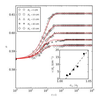
**Figure 5.** Experimental results of the compaction of a glass bead assembly for different initial height. The red lines are the KWW expression (1). Insert: the fitted characteristic time  $\tau$  as a function of the initial volume fraction.
