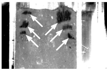
**Figure 7.** Image of the  $\text{UO}_2$  powder during the vibration process. The arrows indicate macro-cavities near the front plate. Only the top of the tank is shown here.
