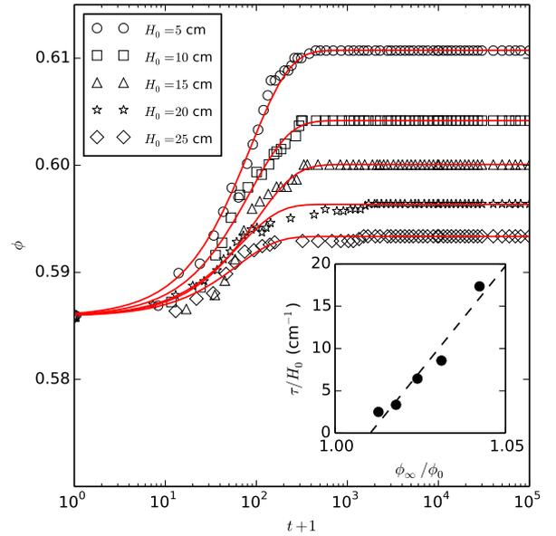
**Figure 5.** Experimental results of the compaction of a glass bead assembly for different initial height. The red lines are the KWW expression (1). Insert: the fitted characteristic time  $\tau$  as a function of the initial volume fraction.
