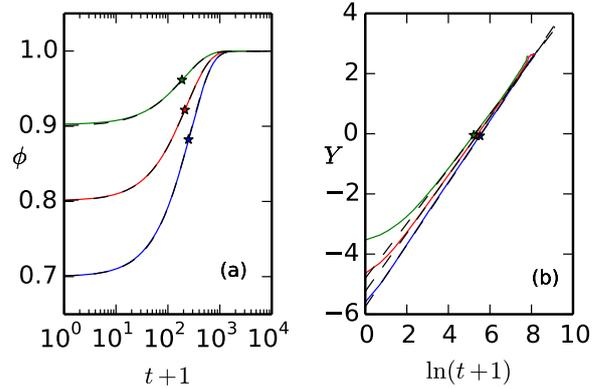
**Figure 3.** Simulation results (colored continuous lines) for  $N = 250$  grains, averaged on 20 000 runs. Each curve is fitted by Eq. 1 (dashed black line) (a) Compaction curves for three different initial conditions. The star symbols indicate the inflexion points at time  $t = T$ , (b) Same data in the  $(\ln t, Y)$  space.
