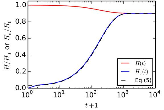
**Figure 2.** Height of the modeled packing  $H(t)$  (red curve) normalized by the initial height  $H_0$ , height of the compacted grains  $H_c(t)$  (blue curve), compared with expression 5 (black dashed line). The model parameters are  $N = 250$ ,  $\phi_0 = 0.9$  from an average of 20 000 runs.
