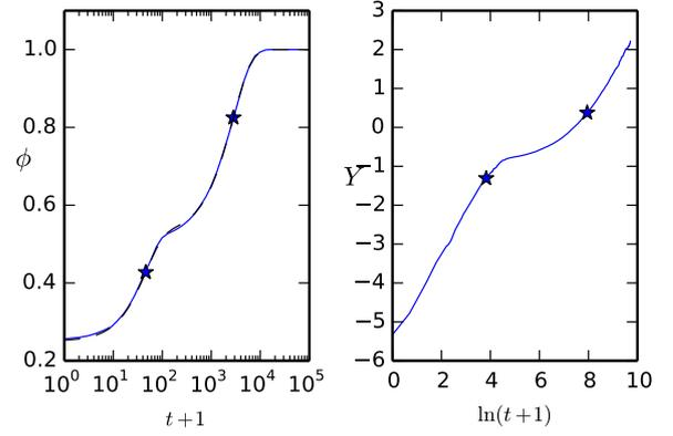
**Figure 4.** Simulation result for a modeled cohesive granular material. The parameters are  $N = 1250$ ,  $n = 50$ ,  $\phi_{0c} = \phi_{0g} = 0.5$ . (a) volume fraction as a function of time in a log-lin space (blue curve) and the fitted expression (12) (black dashed line). The stars indicate the  $T_c$  and  $T_g$  characteristic times. (b) Same data plotted as  $Y = \ln(\ln(1/C))$  as a function of  $\ln t$ .
