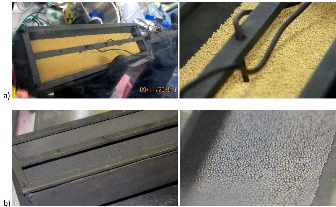
Figure 1: Microspheres a) before calcination under air (total weight~50g) b) after calcination under air 700°C-4h (total weight~22g)
