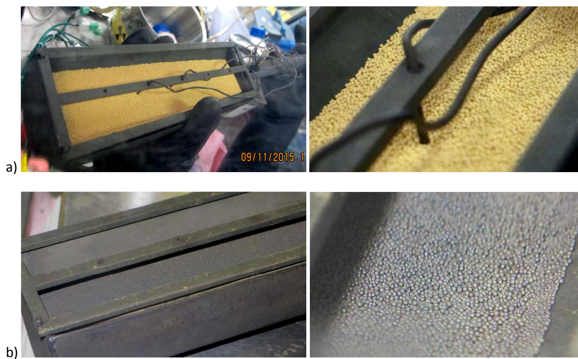
Figure 1: Microspheres a) before calcination under air (total weight~50g) b) after calcination under air 700°C-4h (total weight~22g)
